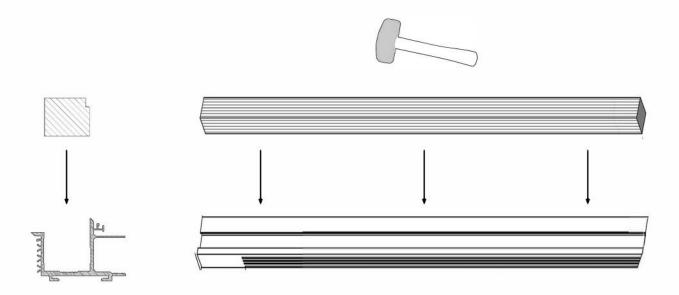
2. ensure that the timber is fully inserted and flush with the top of the frame
