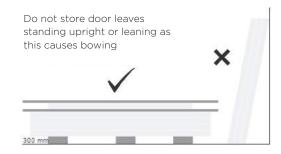
It is important for doors and doorsets to be handled and installed in align with BS Code of Practice, CP 151.
